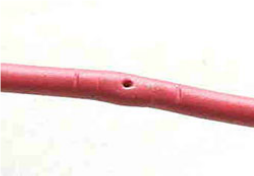
Tapped wire after removal.
