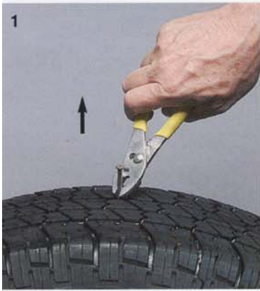
1 Locate puncture and remove damaging item
