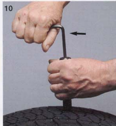
10 Then turn counter-clockwise until inner rod returns to bottom of Plugger
