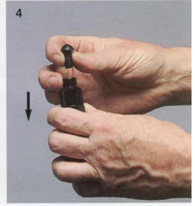
4 Set mushroom plug into Plugger with stem down
