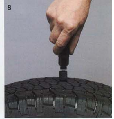
8 Screw loaded Plugger onto nozzle in tire
