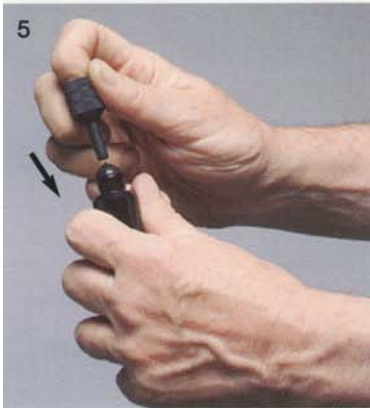
5 Use nozzle to recess mushroom head down into Plugger
