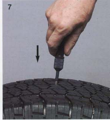
7 Insert probe and nozzle into the hole then unscrew probe from nozzle
